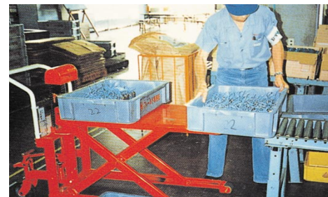
Set at the same height as the conveyor belt and slide things over
